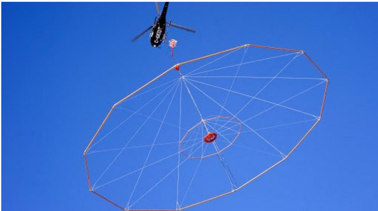
**Figure 1:** VTEM MAX™ system in flight at Halls Creek Project (Photo – Geotech)
