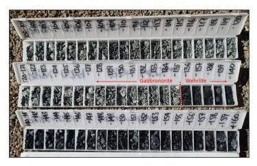
Drill chips from PRRC029 showing mafic-ultramafic contact
