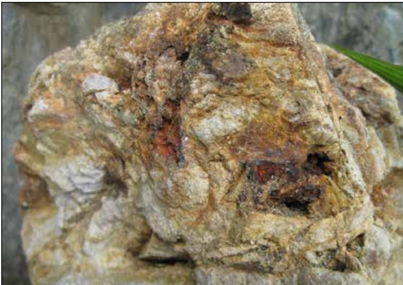
Figure 4-6: Breccia of angular fragments of intrusive and weathered shale with sulphide matrix and sulphide veins
