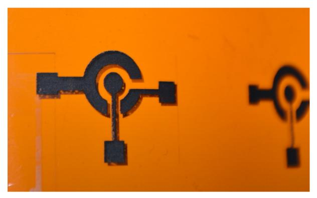
**Fig. 1.** Printed graphene electrodes developed using graphene-based conductive inks derived from Archer's Campoona graphite as part of the collaboration with The University of Adelaide ARC Graphene Hub. Archer and the Partner will use the electrodes as key componentry in the development of a biosensor that can detect diseases.
